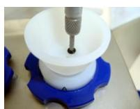
Insert the NO sensor into the stopper with the 2.3 mm additional port. Fix its vertical position by applying a small O-ring on the shaft of the NO sensor (O-rings from old NO sensor sleeves are suitable). The NO sensor should protrude from the stopper by only a few millimetres, low enough to be in a well-stirred zone but high enough not to interfere with the stirrer.
