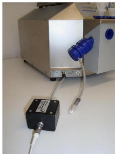
connected to an oxygen channel to obtain simultaneous NO and O<sub>2</sub> recordings.
