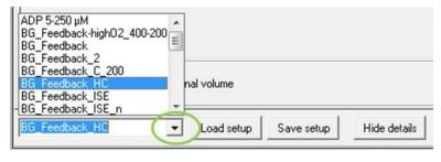
Load setup button will be highlighted in yellow. Clicking on Load setup will then load the new setup into the `TIP2k control' window. Any unsaved changes to the current setup will be lost. The Load setup and Save setup buttons are available from all tabs of the `TIP2k control' window.
