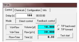
calculated from the two supplied by the user. Select one of the following three options for defining the volume, flow and time (duration) of active pumping:
