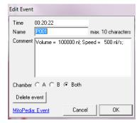
conditions the displayed volume will correspond usually to the injected volume (unless the injection was stopped manually). In feedback mode with using stop condition this initially programmed volume usually will not be reached. The correct volume in this case (and in the case of a manual termination) is displayed in the **PStop** event. Injections are numbered sequentially **P002**, **P003**,... during the entire TIP setup program.
