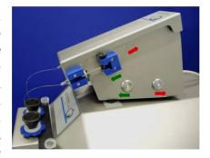
the screw of the syringe plunger pointing towards the side to avoid damaging the syringe and the TIP2k. Of note, when using 500- $\mu L$  microsyringe tighten also the front screw in TIP2k series A or B.
