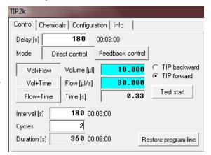
**Interval [s]** is the total time from the start of a pumping cycle to the start of the consecutive cycle. It is the sum of the titration-injection (pumping) "Time [s]", and a pause between the end of the previous and the beginning of the following pumping state.
