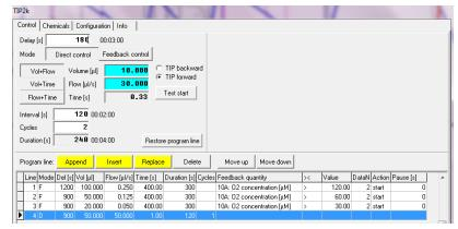
situated between the input mask and the program lines table, and the **program lines table** in the lower part of the window.
