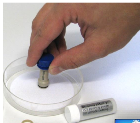
Cathode cleaning on the polishing cloth.
