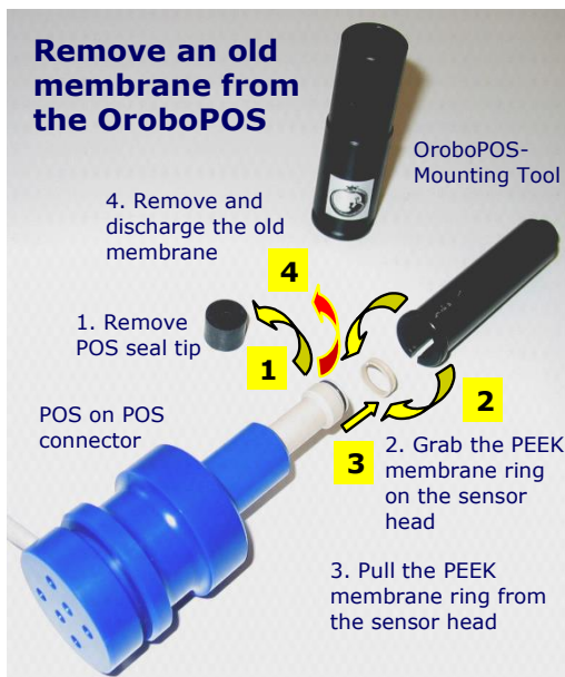
Removal of a used membrane from the OroboPOS.
