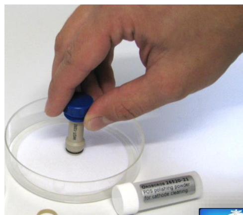
Cathode cleaning on the polishing cloth.
