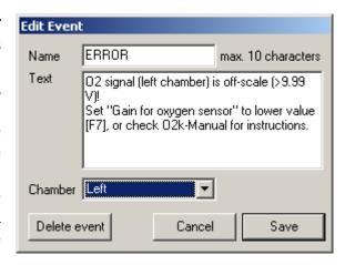
An error message is additionally recorded as an event if the oxygen signal is above 9.99 V for more than 60 s.
