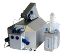
OROBOROS Oxygraph-2k, with Titration-Injection microPump (TIP2k) on top, and the Integrated Suction System (ISS) on the right. lead not merely a system of high quality instruments but distinguish **high-resolution respirometry as a method and concept**. The OROBOROS Oxygraph-2k is the standard instrument where high resolution counts, at low respiratory activities, fast transitions and at low oxygen levels. High resolution is required in particular for the analysis of:
