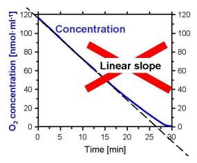
Conventional oxygraphic instruments display merely oxygen concentration over time, and oxygen flux (respiration) is estimated from the slope. Traditionally, linear linear of the experiment sections were analzed using a ruler on the trace of the chart recorder. With this "eyefitting" technique, traces appear to be more linear than they are. The "linear slope" approach belongs to the past of bioenergetics.
