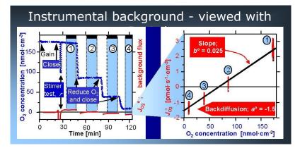
Corrections for instrumental background are an essential standard in high-resolution respirometry, automatically performed by the DatLab software (modified after Gnaiger 2001).
