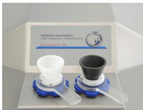
**Stopper-spacers** used for air calibration with white PVDF stopper (Chamber A) or black PEEK stopper (Chamber B).
