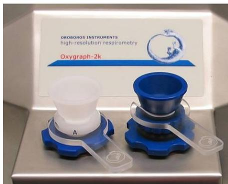
We recommend to replace titanium stoppers with the new PEEK stoppers and corresponding O2k-Chamber holders.
