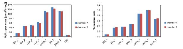
**Fig. 8:**  $O_2$  flux per mass [pmol·s<sup>-1</sup>·mg<sup>-1</sup>] and flux control ratio normalized to PMGS<sub>E</sub> and corrected for ROX, of chamber A and chamber B, in mouse liver homogenate.
