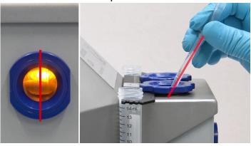
When using the ISS to siphon off solution from the chamber, insert the tip of the ISS to the bottom of the O2k-chamber, pointing it away from you while the stirrer bar is rotating. Do not point the tip towards the oxygen sensor (left and right side in chambers A and B), to avoid damage of the membrane.
