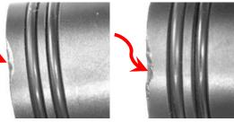
To avoid contamination, hold the stopper at the receptacle, not on the shaft that fits into the O2k-chamber. Do not hold the stopper on the volume-calibration ring when pulling it out from or inserting it into the O2k-chamber, to avoid displacement of the volume calibration position.
