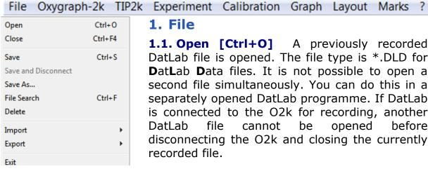
1.1. Open [Ctrl+O] A previously recorded DatLab file is opened. The file type is \*.DLD for DatLab Data files. It is not possible to open a second file simultaneously. You can do this in a separately opened DatLab programme. If DatLab is connected to the O2k for recording, another cannot be opened disconnecting the O2k and closing the currently recorded file.
