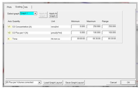
Left mouse click on the X-axis,  $Y_1$ or  $Y_2$ -axes opens the F6 window. The F6 window provides flexibility to vary the display of the plotted data according to specific needs. Viewing plotted data differently scaled graphs, zooming the signal and
