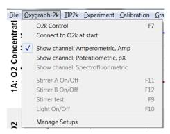
**Oxygraph-2k** Deselect channels ('Show channel') that are not actually recorded. Channels are deselected and shown in grey if no data are available.
