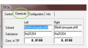
Left/Right refers to the side of the syringes and O2k-Chambers.Solvent is the liquid in which the chemical in the TIP syringe is dissolved.
