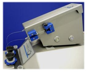
rubber feet of the TIP2k need to be positioned at a 5 cm distance from the front edge (see picture). If you received the TIP2k separately, use the tool for placing the TIP2k-Position marker correctly on the O2k (included in the shipment). Align the rear ends of the TIP2k and the Oroboros O2k. This leaves space for syringe and tube racks.
