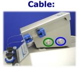
A 0.5 m cable connects the TIP2k to the O2k at the rear, with a 15 pin female SubD plug.
