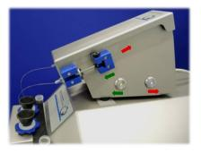
with the step motor of the TIP, for fixation of the plunger. When using 200 µl microsyringes with the TIP2k, tighten the back screw and do not use the front screw. Otherwise the syringe may break. It is important to have the screw of the syringe plunger removed to avoid damaging the syringe and the TiP2k.
