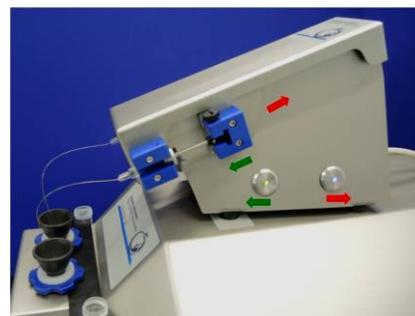
**Push buttons** are located on the right side of the TIP2k. Push the front one (green light) for forwards movement, and the rear one (blue light) for backwards movement of the plunger holder. For stopping the manual movement, simply release the push button. Pushing both buttons simultaneously also stops the pump. At manual operation of the TIP2k, the step motor moves at maximum speed.
